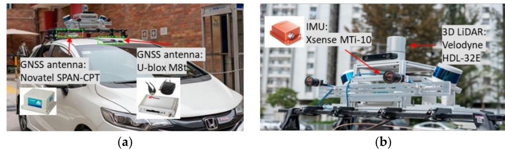
Figure 4. Sensor setup deployment during the experimental data collection. (a). GNSS antennas of NovAtel SPAN-CPT and u-blox M8t. (b). The Xsens Ti-10 IMU and the Velodyne HDL-32E LiDAR.
